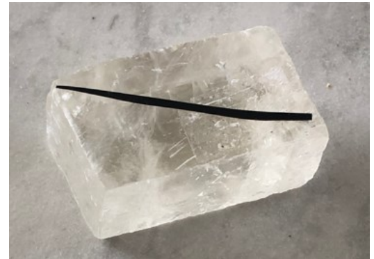
Icelandic spar, also called optical calcite, from Iceland is used in demonstrating the polarization of light with a strip of tape on one side.
