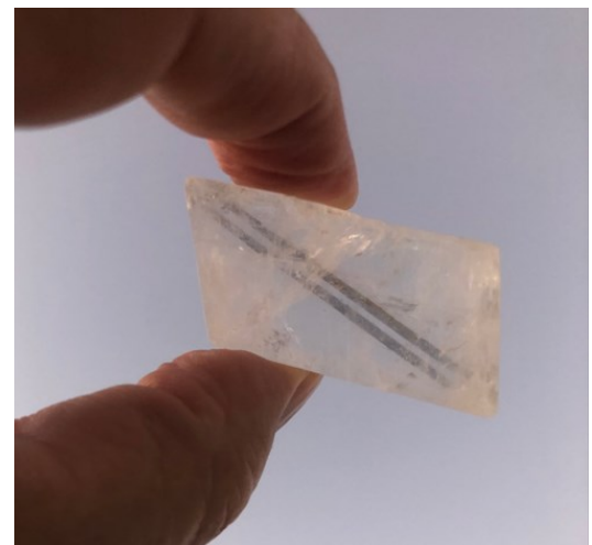
The sunstone pointed in the direction the sun during civil twilight - the projected images are the same shade..
